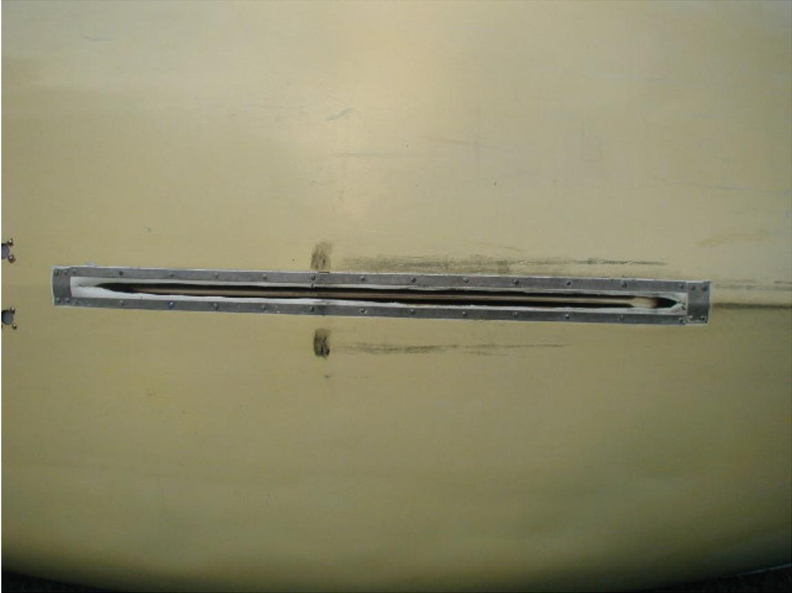
This is a picture of the old rubber gasket that was on my boat when I got it. I'm not sure if it was the original, but I understand that is what Chrysler used back in the "70's. It was extremely worn, and I believe that a previous owner may have cut away a portion of it so that the centerboard would move more freely. With the big gaping hole in the bottom water was splashed up the trunk and into the cockpit.
